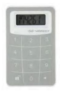
The use of the token (VASCO DigiPass 270) is very simple. Every time that an authorized user wishes to log into iPKO biznes or wants to carry out an operation, he will be asked to enter a code generated by the token. For higher security, the token is protected by a PIN code. At the moment of delivery the PIN code is 12345. When using the token for the first time, the user must change the PIN number.
