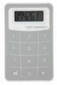
The token (VASCO DigiPass 270) is very easy to use. Whenever an authorized user wishes to log in to the iPKO biznes webste or perform a transaction, they will be asked to enter a code. For greater security, the token is protected by a PIN. On delivery, the PIN is set to 12345. You should change it when you use the token for the first time.
